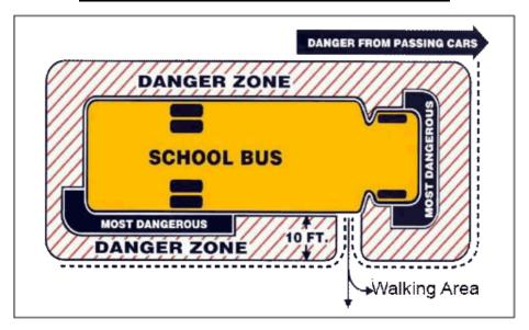
For the safety of students, they should maintain a minimum 10 - 12-foot distance from the sides and front of the bus when waiting for the bus, departing the bus and/or crossing. The 10 feet of area in front of the bus and the 10 feet of area around the bus, are the most dangerous areas of school buses due to limited visibility and blind spots. The driver's side of the bus is an additional danger area due to cars attempting to pass the bus from that side.
